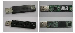
Fig. 5. IronKey D2 before and after epoxy removal
