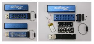
Fig. 41. Datashur Pro before and after opening its metal case
