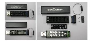
Fig. 46. Datashur before and after opening its metal case
