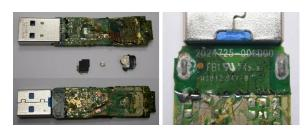
Fig. 24. IronKey D300 after epoxy removal
