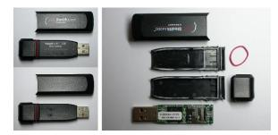
Fig. 48. Stealth M200 before and after opening its plastic case
