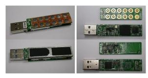
Fig. 44. Datashur Pro2 before and after epoxy removal
