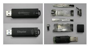
Fig. 23. IronKey D300 before and after opening its metal case
